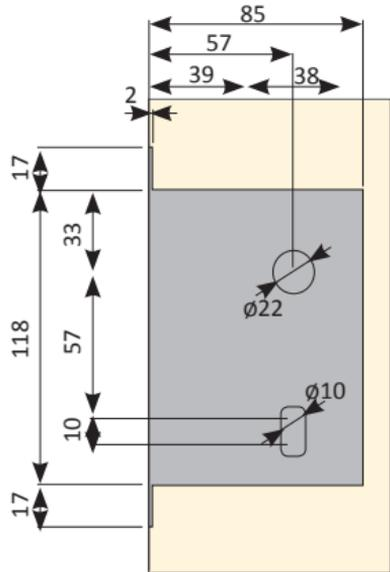
Tools Needed: Drill  $\varnothing$  10mm
